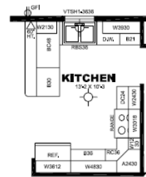
OPT. KITCHEN 1/4"=1'-0" (DIMENSIONS FRAMING TO FRAMING)
